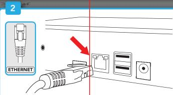
Plug one end of the included Ethernet cable into the LAN port on the back of the WNVR.
