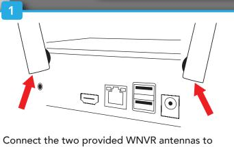
the antenna ports on the rear of the recorder.
