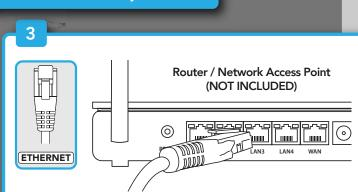
Plug the other end of the Ethernet cable into a port on the back of your router / network access point.
