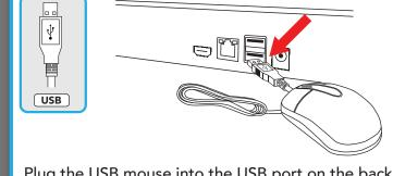
Plug the USB mouse into the USB port on the back of the WNVR.
