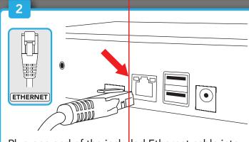
Plug one end of the included Ethernet cable into the LAN port on the back of the WNVR.
