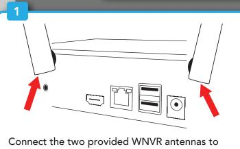
the antenna ports on the rear of the recorder.
