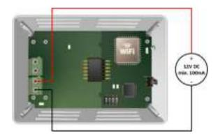
Important: If a wired remote controller of the AC manufacturer is connected in the same bus, communication may shut down. In case it happens, use an external power supply connected to the PS connector in our device to overcome this situation. Connect a NEC Class 2 or Limited Power Source (LPS) and SELV rated power supply to the device, respect the polarity. Apply always a voltage within the range admitted and of enough power (12V DC, min. 100 mA).
