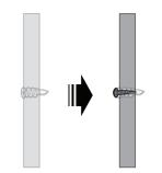
Insert the screws into the holes and tighten the screws until only 1/4 inch of the screws are exposed.
