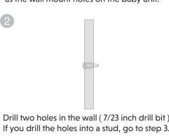
If you drill the holes into a stud, go to step 3. If you drill the holes into an object other than
