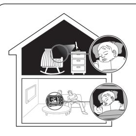
The baby unit has infrared LEDs that allow you to see your baby clearly at night or in a dark room. When the baby unit being viewed detects low light levels, the infrared LEDs are switched on automatically. The images from the baby unit are in black and white, and 2 ppears on the screen.
