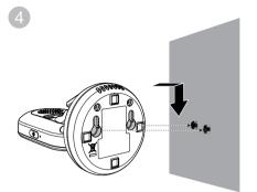
Align the wall mount holes on the baby unit with the screws on the wall. Slide the baby unit down until it locks into place.
