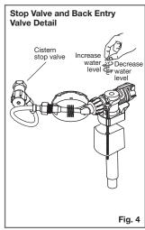
Note: The inlet valves are suitable for dynamic flow pressures of 30 kPa to 1000 kPa.
