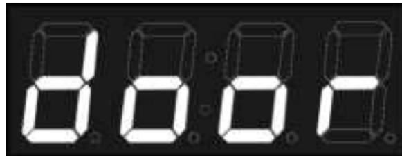
Figure 27. Door open indicator
