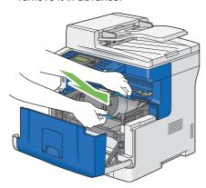
3 Make sure that the two tabs of the toner cartridge align with the grooves on the printer, and then insert it into the printer until it clicks.
