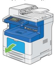
4 Grasp both sides of the bypass tray, and then pull the bypass tray from the printer.
