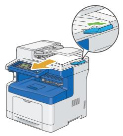
3 Remove any paper in the output tray and slide the output tray extension inside the printer.
