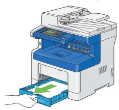
4 Hold the standard 250 sheet tray with both hands, and remove it from the printer.
