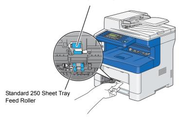
7 Insert the standard 250 sheet tray into the printer, and push until it stops.
