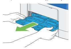
4 Pull the tray out of the printer about 200 mm.
