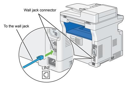
To connect a telephone and/or answering machine to your printer, plug the telephone or answering machine line cord into the phone connector ( ).
