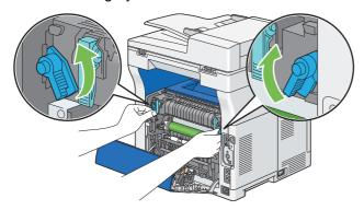
4 Grasp the grips on both sides of the fusing unit placing thumb on the knurling, and then pull out the unit.
