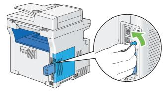
4 Slide the control board cover towards the rear of the printer and remove the cover.
