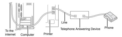
If you want to use your computer modem for faxing or for a dial-up internet connection, connect the computer modem directly to the rear of your printer with the TAD as shown above.
