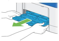
7 Pull the standard 250 sheet tray out of the printer about 200 mm.
