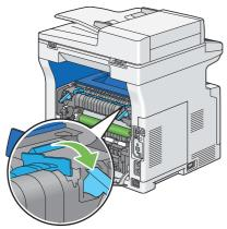
**b** Remove the jammed document from above the fusing unit.
