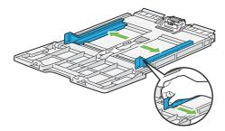
4 Pull up the length guide and slide it toward the bypass tray cover until it stops.
