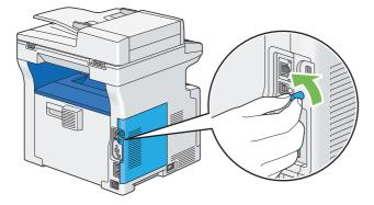
3 Slide the control board cover towards the rear of the printer to remove the cover.
