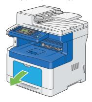
6 Grasp both sides of the bypass tray, and then pull the bypass tray from the printer.
