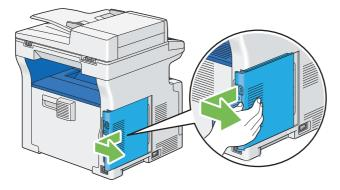
5 Remove the wireless printer adapter from the printer by releasing the adapter's hook while pushing the wireless printer adapter towards the front of the printer.
