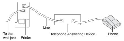
You can connect a telephone answering device (TAD) directly to the rear of your printer as shown above.
