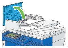
**b** Lift the release lever 90 degrees and remove the jammed document by carefully pulling the document in the direction of the arrow shown in the following illustration.
