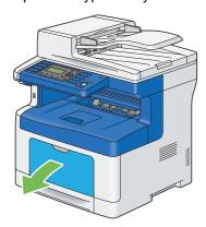
2 Grasp both sides of the bypass tray, and then pull the bypass tray from the printer.
