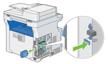
6 Align the guide on the control board cover with the slot around the control board, and slide it towards the front of the printer.
