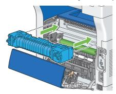
4 Lower the two gray levers to lock the fusing unit.
