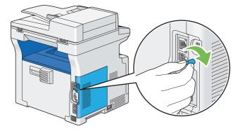
8 Reconnect all cables into the rear of the printer and turn on the printer.
