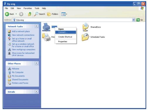
Wait for the driver information to be copied from the server computer to the client computer, and for a new printer object to be added to the **Printers and Faxes** folder. The copy time varies, based on network traffic and other factors.
