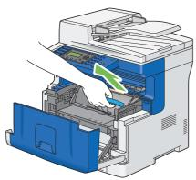
4 Grasp the handle on the front of the drum cartridge, and then pull it out halfway with one hand.
