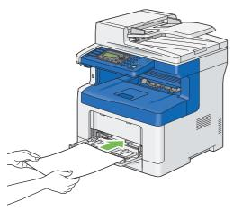
4 Slide both width guides until they rest lightly against the edge of the print media stack.
