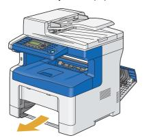
7 Insert the standard 250 sheet tray into the printer, and push until it stops.
