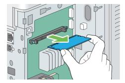
6 Align the guide on the control board cover with the slot around the control board, and slide it towards the front of the printer.
