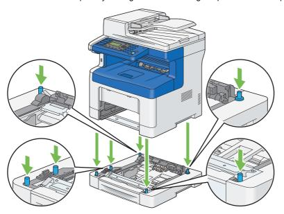
Secure the optional 250 sheet feeder to the printer by tightening the two screws provided with the feeder with a coin or similar object.
