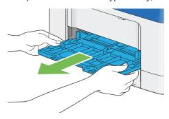
3 Pull the standard 250 sheet tray from the printer about 200 mm.
