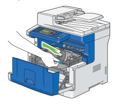
5 Grasp the handle on the top of the drum cartridge with the other hand, and then pull it out completely.
