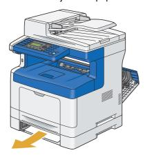
5 Insert the optional 250 sheet feeder into the printer, and push until it stops.
