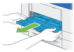
5 Pull the standard 250 sheet tray out of the printer about 200 mm. Hold the standard 250 sheet tray with both hands, and remove it from the printer.
