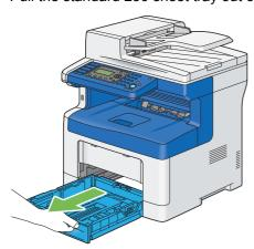
8 Hold the standard 250 sheet tray with both hands, and remove it from the printer.
