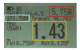
You can then read the TX Power level (red rectangle) and VSWR (orange rectangle) The reading should not exceed 1:5. You will also be able to see the Transmit Frequency (light blue rectangle).
