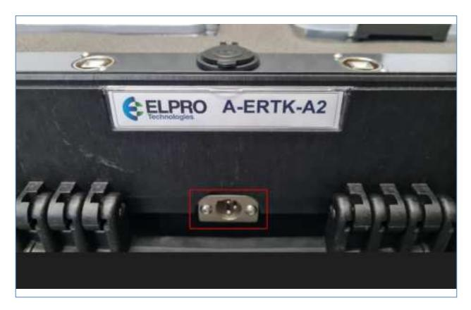
**Charging Port** – Charges the ERT-A2 Receiver /Decoder and the VSWR Meter (if connected to the USB Charging socket)
