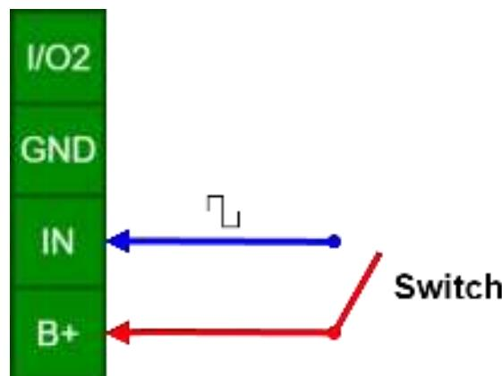
If the sensor has IO2, an analog read will be performed on I/O2 (see 4.2.1) after the pulse frequency is measured. The intended use is passive wind sensors, which commonly have a potentiometer-based wind direction meter.
