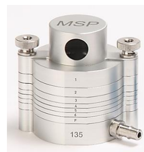
Figure 2: 135-6B MiniMOUDI™ Impactor, with optional cowl inlet installed
