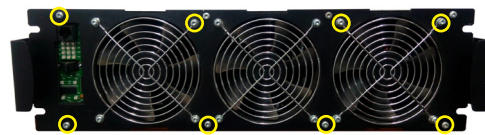
Figure 2: Remove FAN Kit
