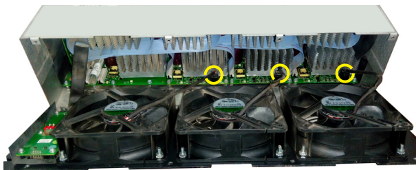
Figure 3: Disconnect the fan wires
