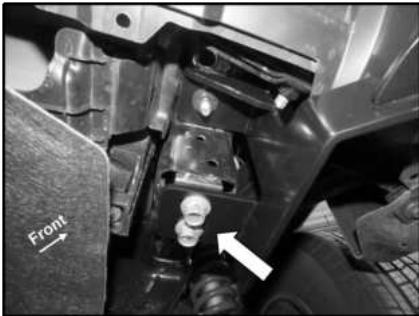
(Fig 4) Complete installation of the Mounting Brackets by reusing the OEM hardware as pictured.
