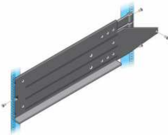
Figure 3. Attach the Mounting Rails to the Rack
