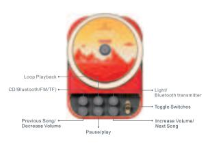
Push [Toggle Switches] up ---- to power on. Turn [Toggle Switches] down ---- to power off. After the device is turned on, there is no operation screen. After 1 minute, the screen will break (enter low power mode).
