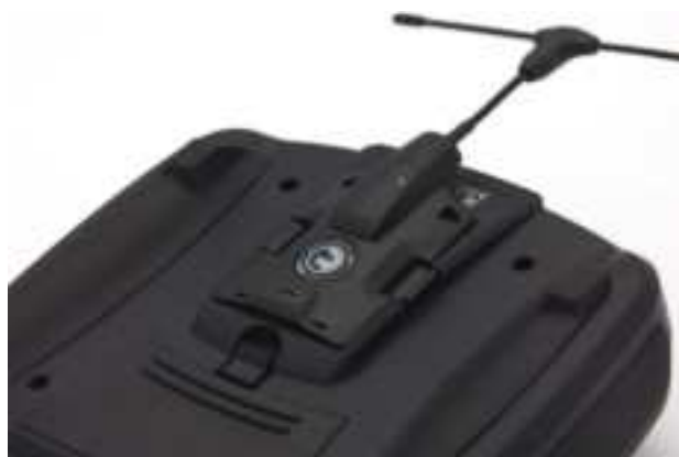
JR bay with installed TBS Crossfire module
