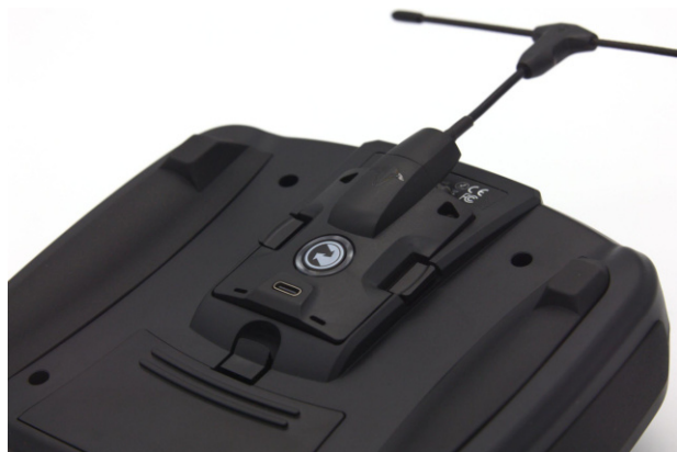
JR bay with installed TBS Crossfire module
