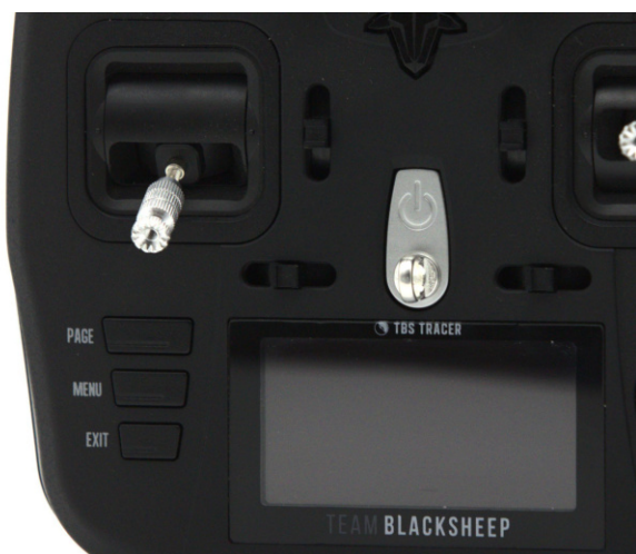
Power button, Left gimbal, Display and speaker
