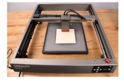
3. Adjust the focal length of the laser module with the multi-level fixed focus block.
