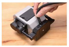
2.2 Plug the air pump cable into the air pump interface on the left side of the machine, and you can adjust the airflow through the knob switch.
