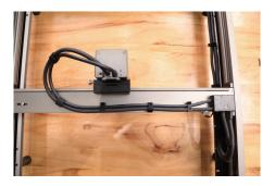
5. Organize the laser module cable and silicone tube with the cable straps.
