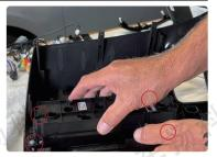
2 Install the knob kit in the designated positions, then mount the air conditioning vent onto the new frame, tighten the three screws on both sides, and proceed to connect the wiring between the new radio and the original vehicle.
