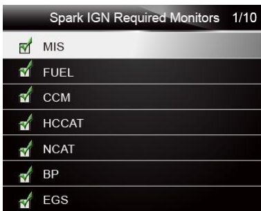
Figure7-6 Sample Spark IGN Required Monitors Selection Screen
