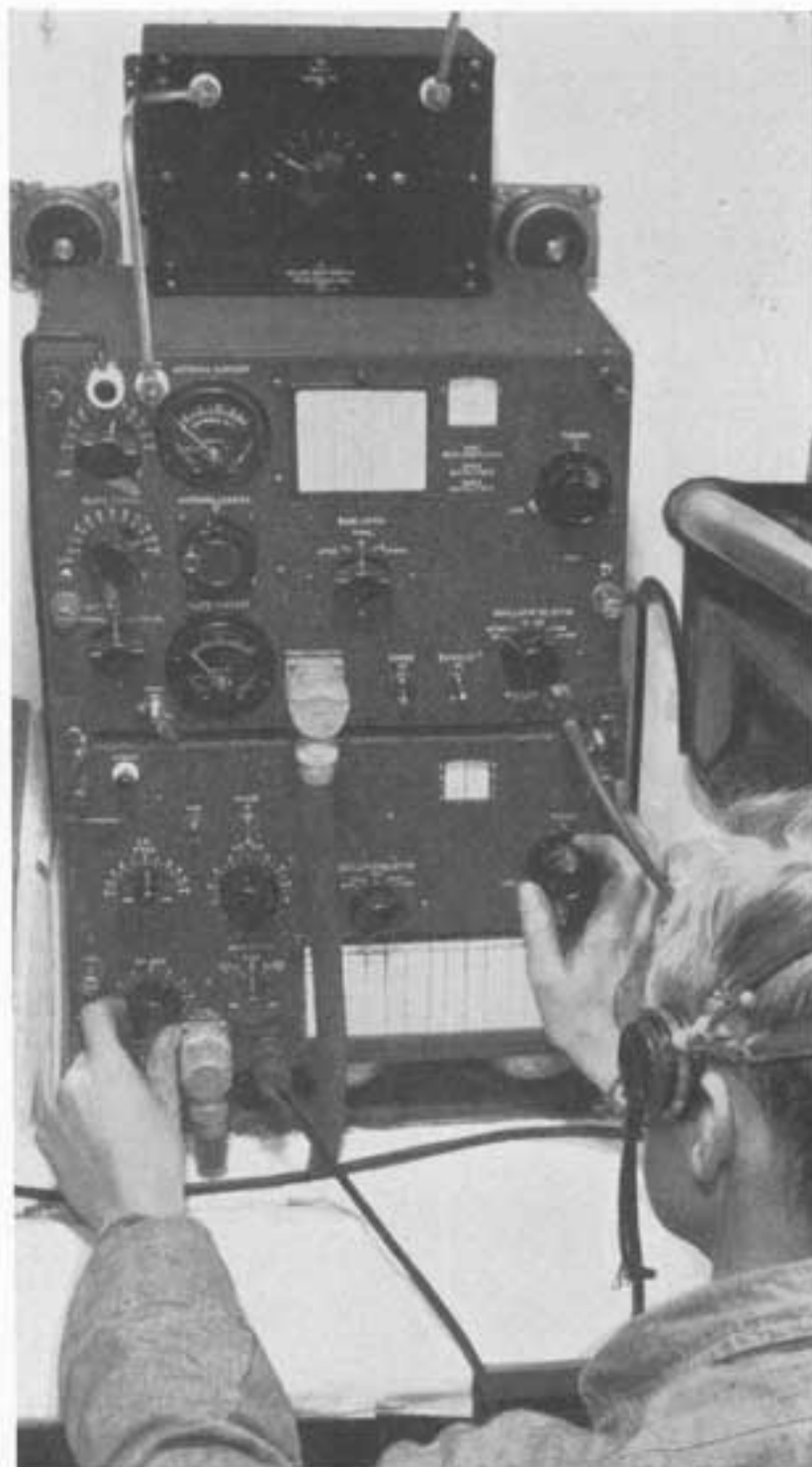
Model TCS transmitting-receiving equipment set up for operation. The antenna loading coil is mounted on top of the transmitter.
