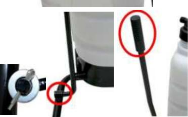
5. The next step is to secure the other end of the connecting rod to the top of the pump. Firstly, insert the pump's lever holder into its position at the top of the pump. Whilst doing this slide through the connecting rod so that it passes through the lever holder as well as the holes on top of the pump. These are secured using the second split pin. Use the photos to help.
