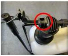
6. Lastly, just place the filter into the filling point. This prevents anything other than liquid entering the tank.
