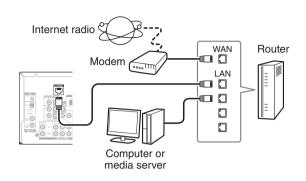
The AV receiver supports Wi-Fi, and you can connect the AV receiver to your home network by wireless LAN. For wireless LAN connection, see "4. Performing Wireless LAN Setup" (→Page 5).
