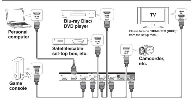
The components connected to each terminal (BD/DVD, GAME, etc.) can be selected with the input selector buttons of the same name on the front panel. Note that these default assignments can be changed. For details, please refer to the instruction manual.
