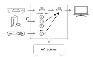
If you've connected your TV to the AV receiver with an HDMI cable, composite video and component video sources can be upconverted and output by the HDMI OUT MAIN.
