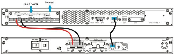
Step 2: Switch the breaker on EBC to "ON" position;
