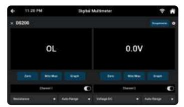
4. Each channel offers a range of measurement options in the Meter Measurement Menu, including Current, Voltage, Resistance, AMP Clamp Meter Mode, Diode Drop, and Continuity. It's important to note that different measurements necessitate specific setups.
