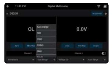
**6.** The "Zero" function facilitates easy calibration of the current reading to zero (0), serving as a reference point for all subsequent measurements and eliminating offset values.
