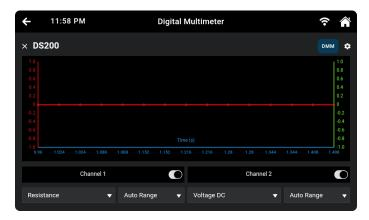
Likewise, the Scopemeter feature merges data from both channels into a cohesive graph, effectively illustrating the interaction between the two parameters.
