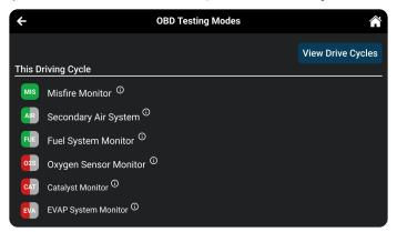
The page refreshes to display the Drive Cycle procedure for the Incomplete or Enabled monitors.
