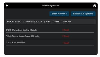
Each report begins with a vehicle information bar that includes a **Report ID**, the vehicle's description (**year/make/model**), the last six digits of the Vehicle Identification Number (**VIN**) and the odometer reading (**ODO**) at the time the scan was performed.
