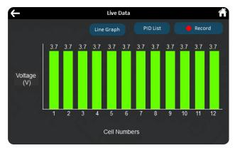
6. The Line Graph button displays battery voltage PIDs in line graph format.
