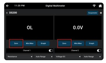
7. The Min/Max function automatically logs the highest and lowest values during the measurement period, eliminating the necessity for manual tracking.
