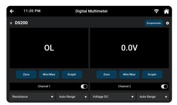
4. Each channel offers a range of measurement options in the Meter Measurement Menu, including Current, Voltage, Resistance, AMP Clamp Meter Mode, Diode Drop, and Continuity. It's important to note that different measurements necessitate specific setups.
