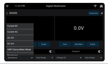
5. In terms of measurement range settings, users can either manually choose their desired range or opt for the **Auto**Range feature. This simplifies configuration adjustments and improves accuracy.
