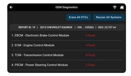
The results window lists all tested Control Modules with its corresponding result:
