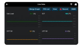
**NOTE:** The Graph function button will stay inactive if the selected PID does not report a numerical value. An example is the Fuel System Status PID, which reports either Open Loop (OL) or Closed Loop (CL).
