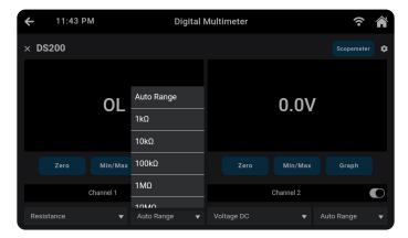
**6.** The "Zero" function facilitates easy calibration of the current reading to zero (0), serving as a reference point for all subsequent measurements and eliminating offset values.
