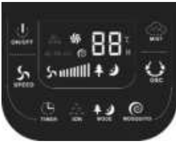
Panel de control
