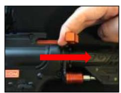
5. GRIP CHARGING HANDLE AND PULL FIRMLY TO REAR TO COCK LAUNCHER UNTIL IT CLICKS, THEN RELEASE
