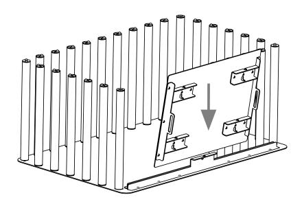
10. Align the holes on the top plate (B) with the bar (D) rivet heads.
