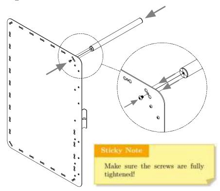
7. Repeat step 4-6 until all bars (D) are fastened to the bottom plate (A).
