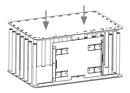
11. Using the allen wrench (G), install a screw (E) to fasten the parts together.
