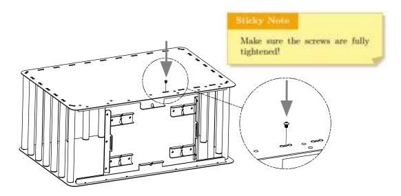
12. Repeat step 11 until the top plate (B) is fastened to the bars (D).
