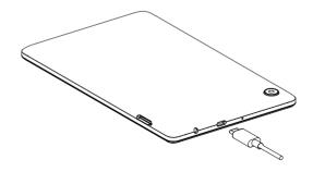
You are advised to fully charge the battery (F3). Charging status is indicated by a percentage displayed on screen. The percentage increases as the tablet is charged.
