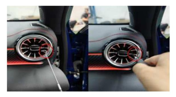
Hook the black frame inside the air outlet and pull back out of the air outlet (as shown)
