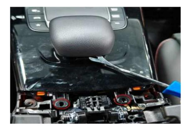
Remove the screws in the red circle and pry open the handle
