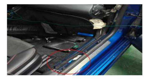
Remove the passenger threshold bar from here (as shown)
