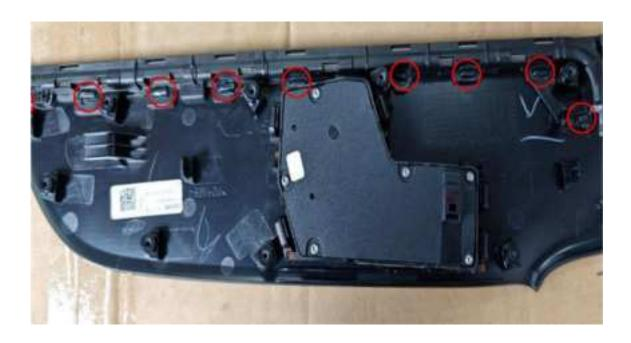
Cut the solder joint, reinstall and weld the atmosphere lamp holder (as shown)
