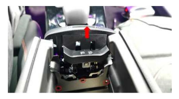
Use the tool to push the buckle into these three holes, press and hold the button to pry up the armrest lid (as shown in the picture).
