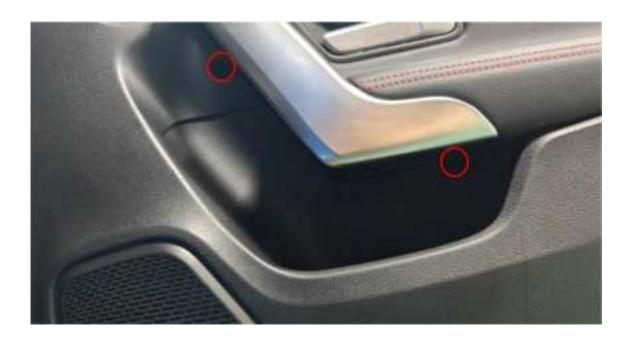
Pry open the cover plate and remove the screw to remove the door panel (as shown in the picture)
