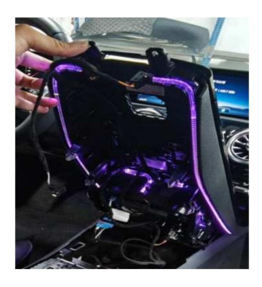
Tilt up the entire panel and install the lamp (as shown)
