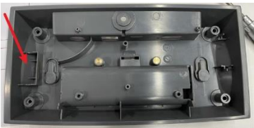
Fix the ferrite core on housing
