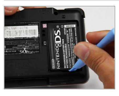
Use a plastic opening tool or spudger to pry out the battery from the bottom. If a plastic opening tool or spudger isn't available, your fingernails may work.
