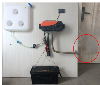
Excessive pump oil produces white smoke
