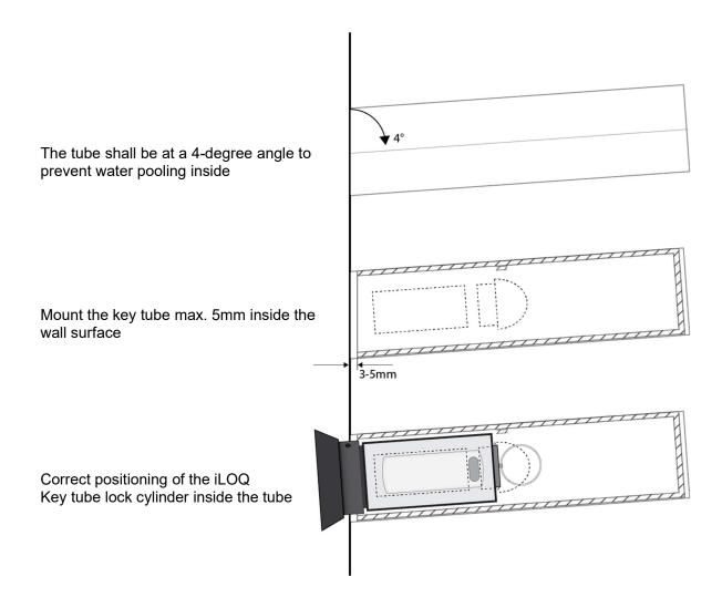
In case an existing key tube is mounted too deep inside the wall and the iLOQ Key tube cylinder cannot be placed in the key tube, it is possible to replace it with a version with a longer version. Please refer to the instructions on the next page and the documentation of the key tube manufacturer.
