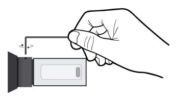
**4.** Tighten the screw by using the 1.5 Nm torque. Ensure that the head of the screw goes into the hole completely. A visible cap indicates that the screw is not in the right place
