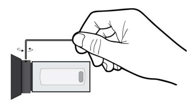
1. Loosen the knob screw by using the TORX 10 tool
