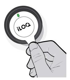
2. Turn the lock-reader knob to unlock the key tube cylinder.
