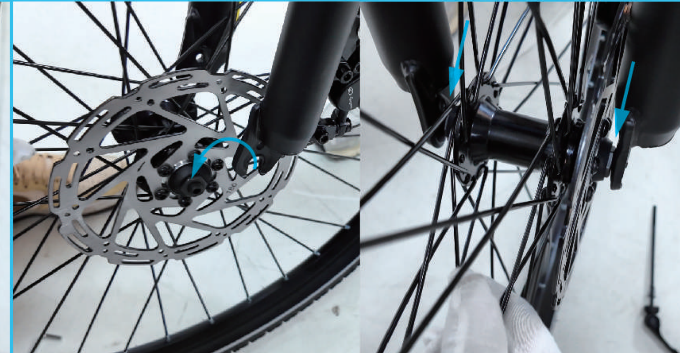
03 Fix the front fork to the designated position of the front wheel (as shown in the figure)
