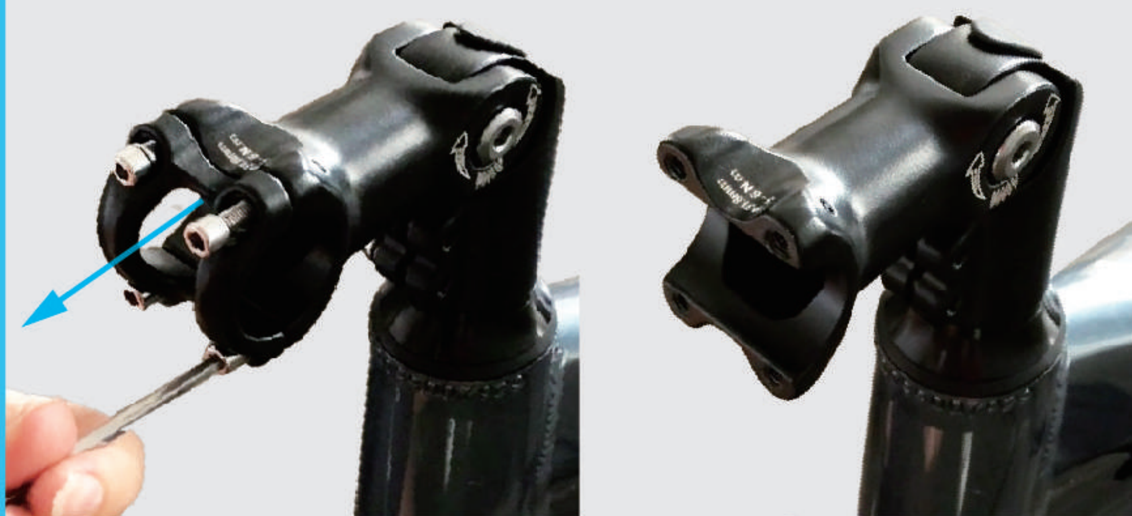
01 Remove the four screws.
