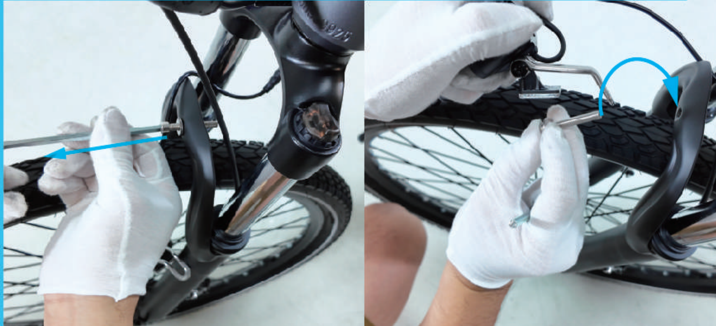
01 Remove the screws here and secure them to the headlight bracket.
