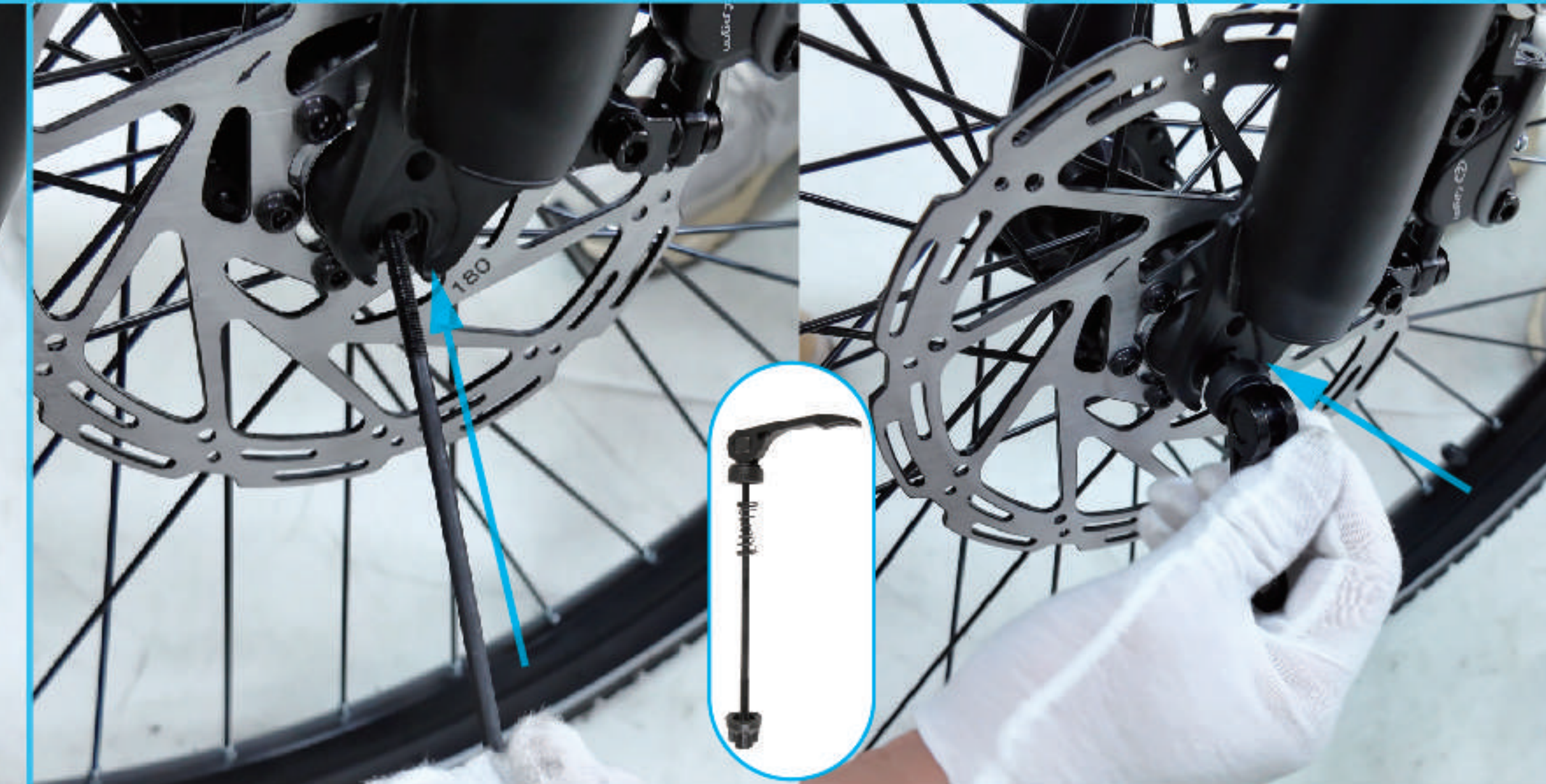
04 Install the quick release shaft and fix the front fork and front wheel. (As shown in the picture)
