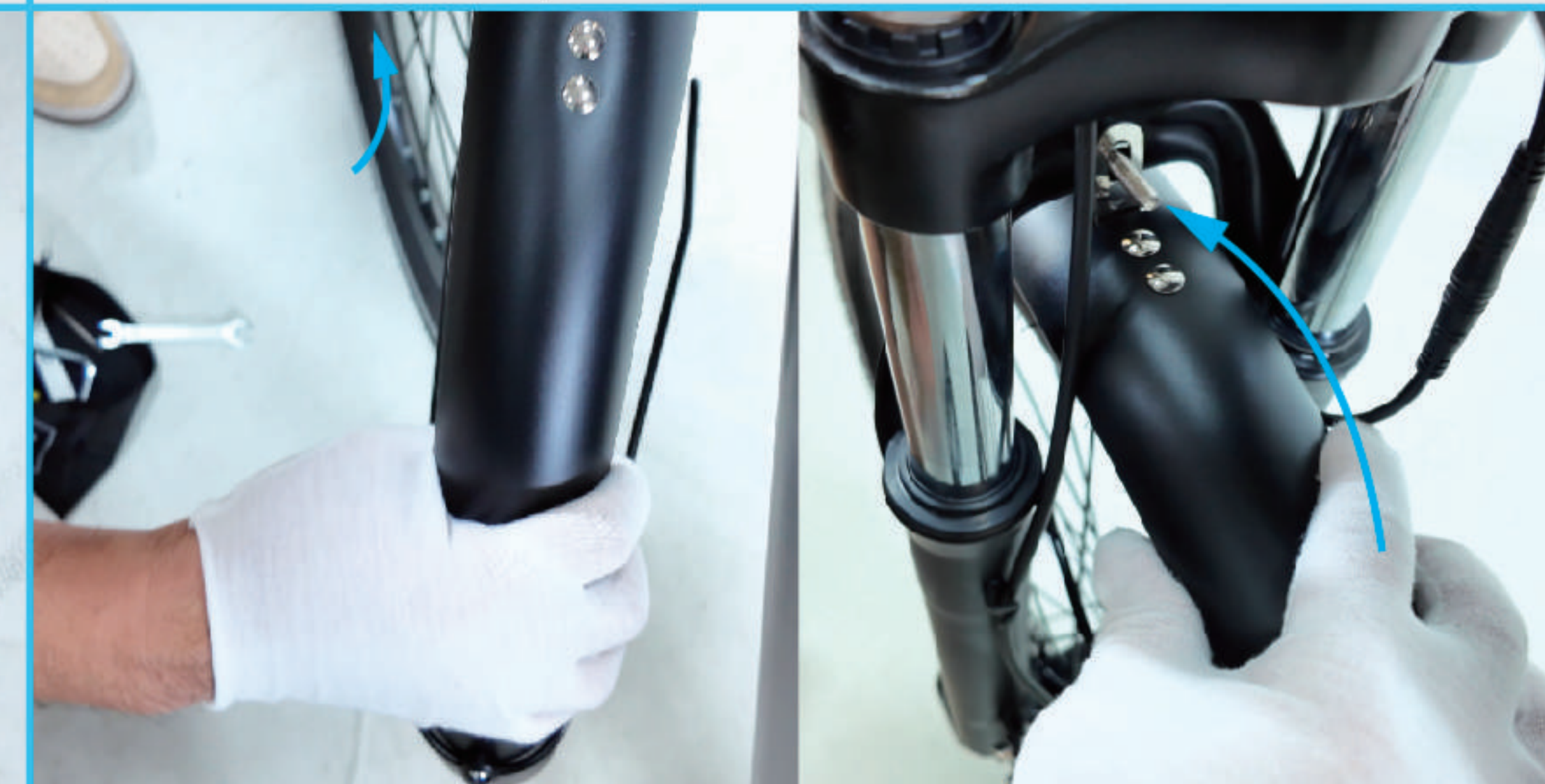
04 Insert the fender into the screws here.
