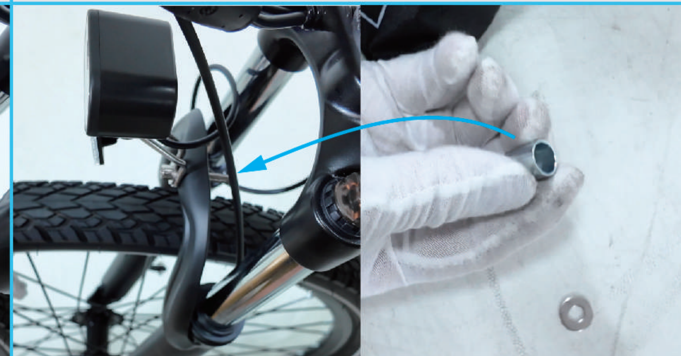
03 After the headlight is fixed, install the fender raising washer. (As shown in the picture)
