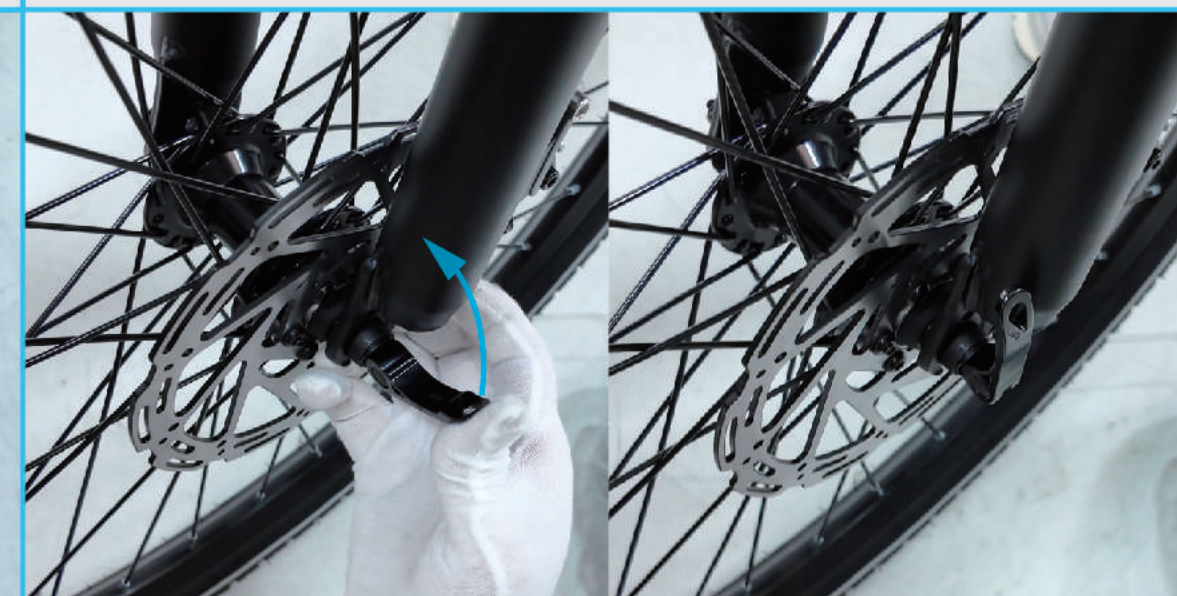
08 Once you are sure the front wheel is in the correct position, lock the quick-release axle to lock it.
