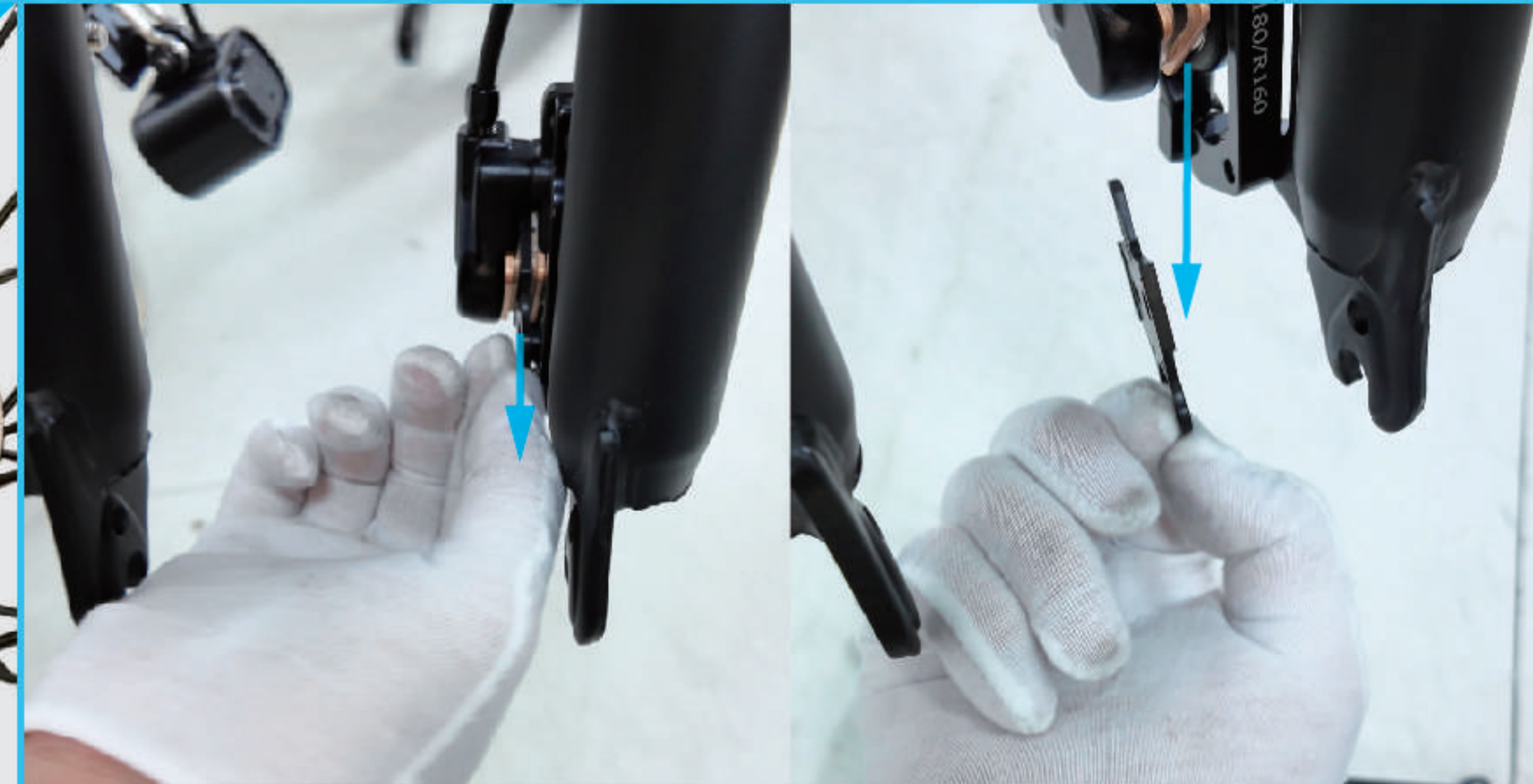
02 Remove the protective shims from the brakes.
