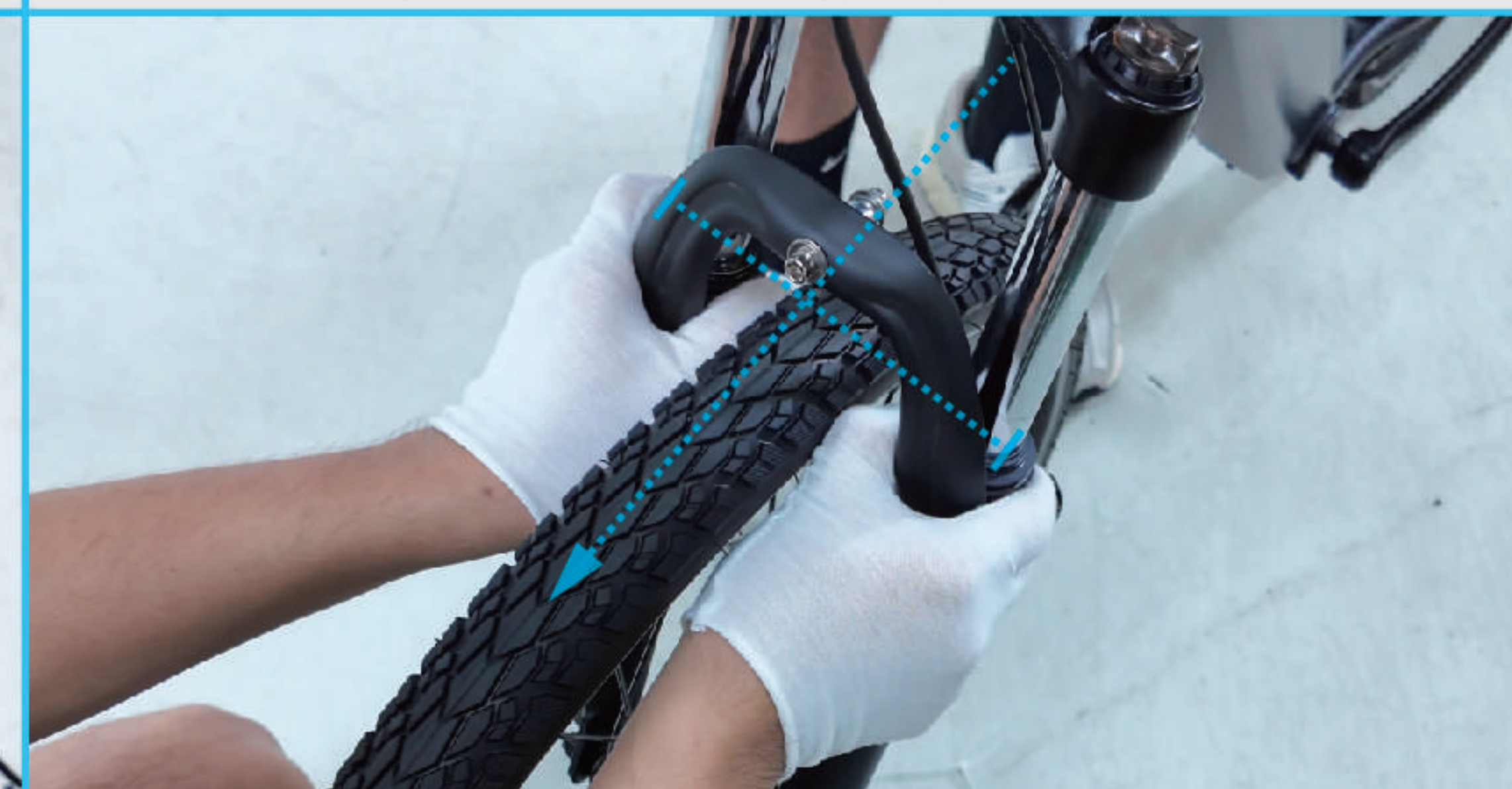
07 Check that the front wheel is centered.
