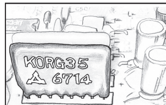
Figure 6: PS-3300 sound generator circuit board, on which the KORG35 was mounted
