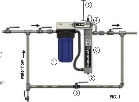
The UV disinfection system should be the last step of your water treatment system. If your water treatment chain involves a pump and pressure tank the UV should be after the pressure tank, not between the pump and tank. Your UV system should be installed after all other water treatment equipment, before the plumbing splits into hot and cold.
