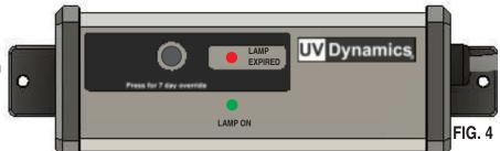
**UV Ballast Start-Up Sequence:** When AC power is applied to the UV power source the lamp is lit as indicated by the green 'LAMP ON' LED. The ballast performs a self-test of the 'LAMP EXPIRED' LED and alarm buzzer consisting of three buzzer beeps and three red LED flashes. If a solenoid is connected to the UV power source it will activate on completion of the self-test sequence.
