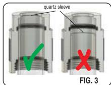
6 Slide glandnut and quartz sleeve into the opening at the top of the chamber and hand tighten firmly. Do not use tools to tighten; overtightening can cause leaks. Do not use any teflon tape, grease, or pipe dope on glandnut threads.
