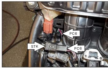
9 Attach the ground wire of the PC6 to the common ground location on the left side of the frame.
