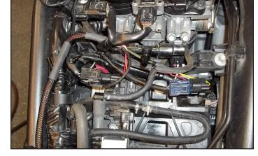
Plug the PC6 harness in-line of the stock TPS and wiring harness.
