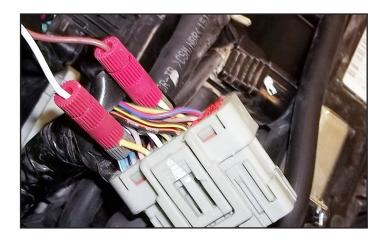
11 Using the supplied Positaps connect the crank wires from the PC6 to the stock wiring harness.
