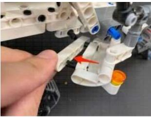
12.) Thread the LED end of a new White 30cm Bit Light down the following space, then connect the connector end of the cable to a new 6-Port Expansion Board.
