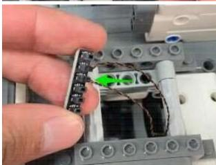
Secure the Bit Light cable in between the following pieces.
