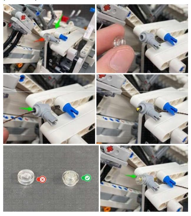
Thread the cable through the inside hole then pull it up toward the back.
