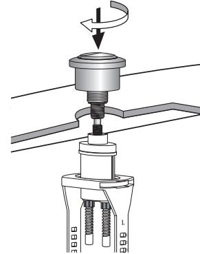
3c. Cover the lid of tank screw the kcy stoke into the thread of the bracket. Check and assure the function of push button is normal without any inieforence.
