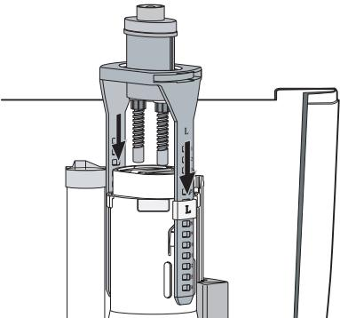
1c. Insert the bracket into the according position of the flush valve and adjust its height as the requirement.
