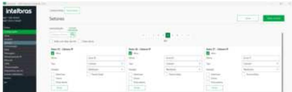
The sector will be triggered when the camera or associated recorder detects the intelligence previously configured in its interface. At the time of triggering, the trigger event will be sent to the monitoring system.
