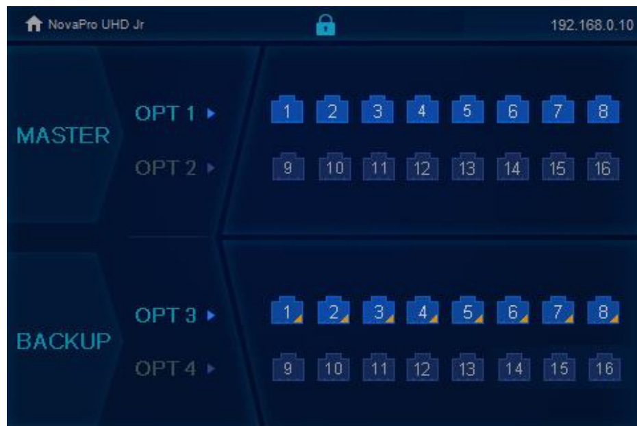
Figure 4-3 Optical fiber port statuses – Hot backup
