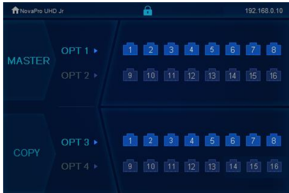
Figure 4-2 Optical fiber port statuses – Copy
