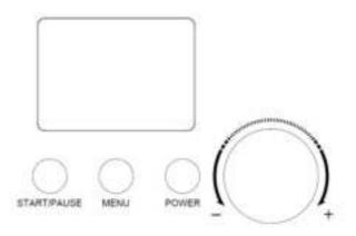
**[POWER]:** After power up, the machine enters standby mode. Then press the **[POWER]** button to enter the setting mode, and LCD will display "60: 00". Press the **[POWER]** button during setting mode, the machine will enter the standby mode again.
