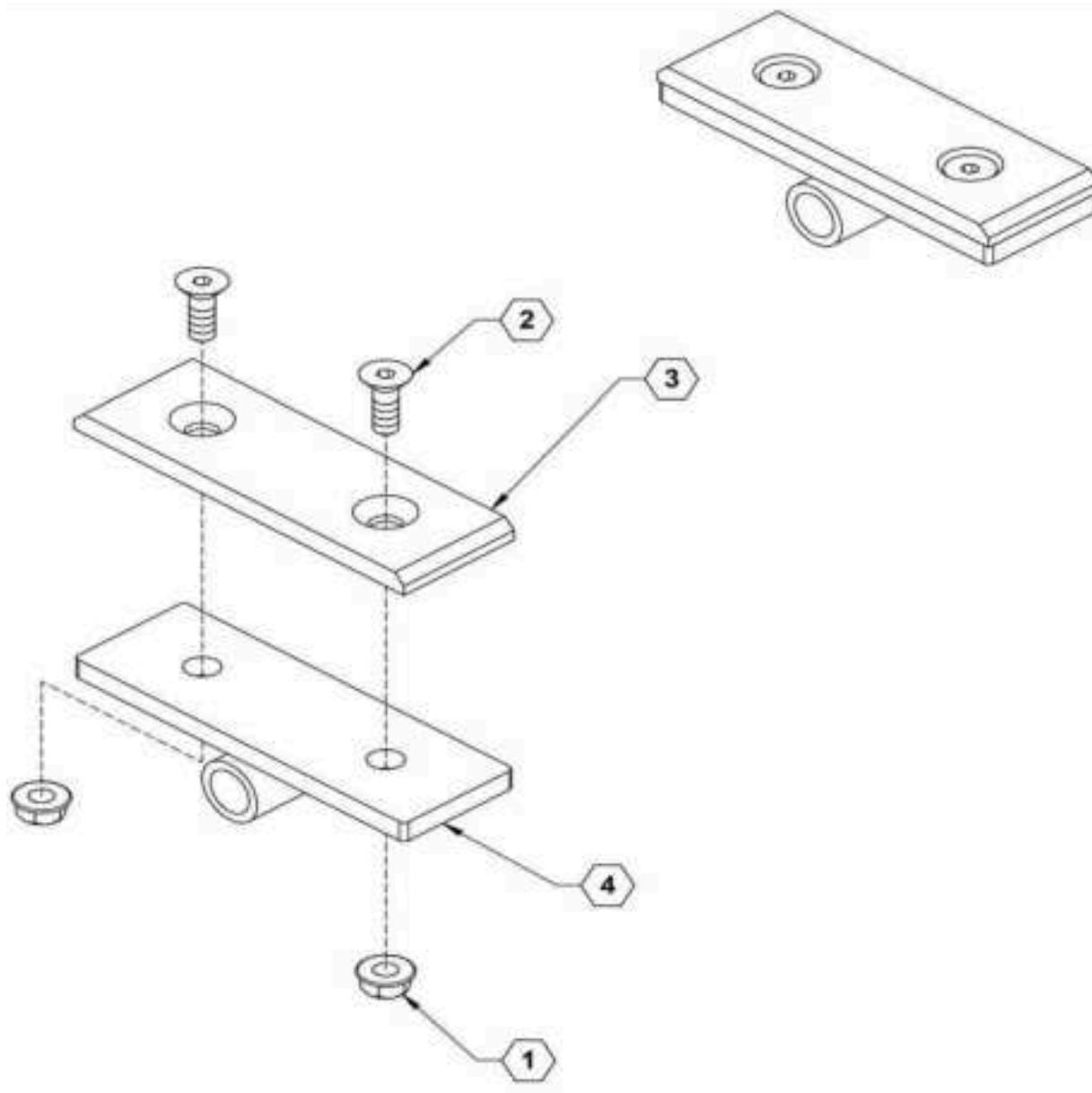
**Parts List 28090: Depth Adjustment Slide Pivot**
