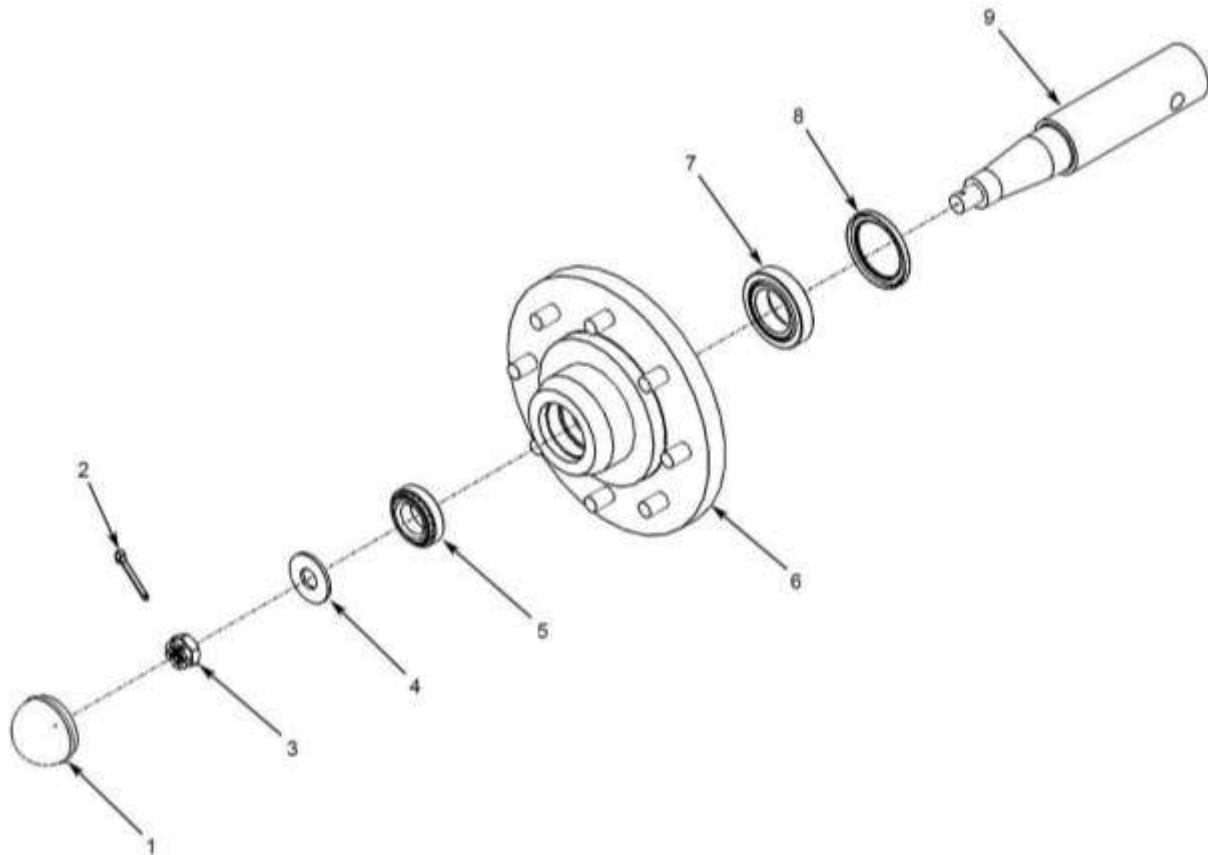
**Parts List 730008: Hub Assembly, 8-Bolt N45-8 (for Main Trailer Wheels)**
