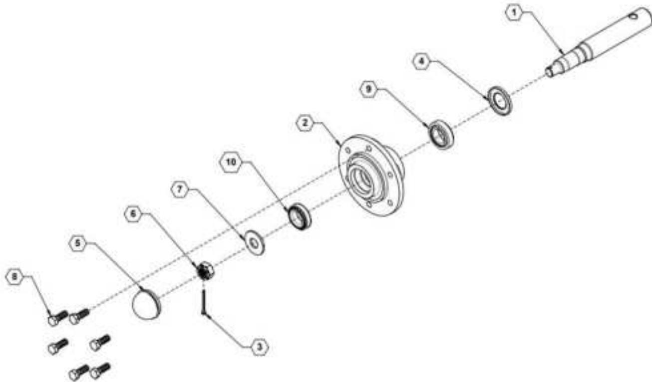
**Parts List 730140: Hub Assembly, 6-Bolt N709 (for Main Trailer Pivot)**
