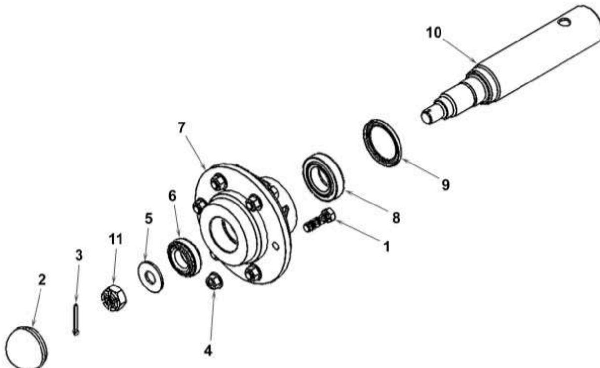
**Parts List 730113: Hub Assembly, 6-Bolt N890 (for Wing Wheels)**
