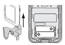
Replace batteries in your indoor sensor when a warning appears on the thermostat screen, about 60 days before batteries are depleted. When the sensor status light begins flashing red, battery power is critically low and will be depleted within 2–3 weeks. During normal operation, the status light remains off.
