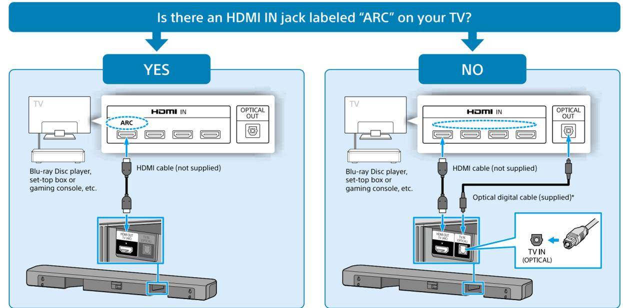
\* If your TV does not support the ARC (Audio Return Channel) function, connect an optical digital cable (supplied) to listen to the TV sound.
