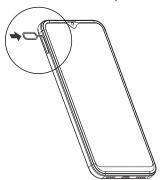
Put 1 or 2 nano-SIM cards onto the SIM tray with the gold contacts facing down and the notched edges match the positions on the SIM tray.
