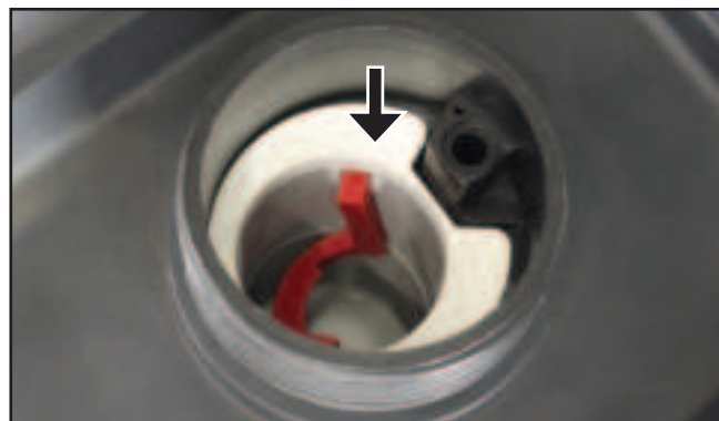
Figure 31 – Reinstalling the Fuel Strainer
