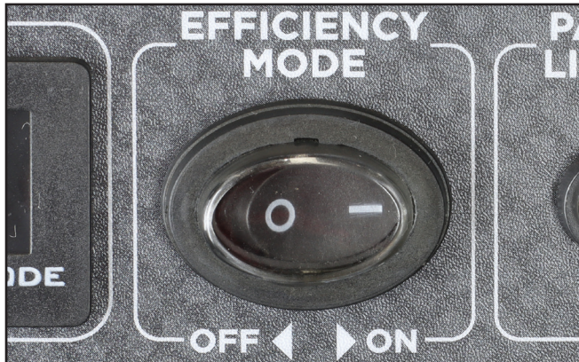
Figure 16 – ECO Throttle Switch in the ON Position
