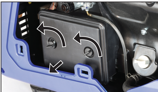
Figure 26 - Removing the Air Filter Cover
