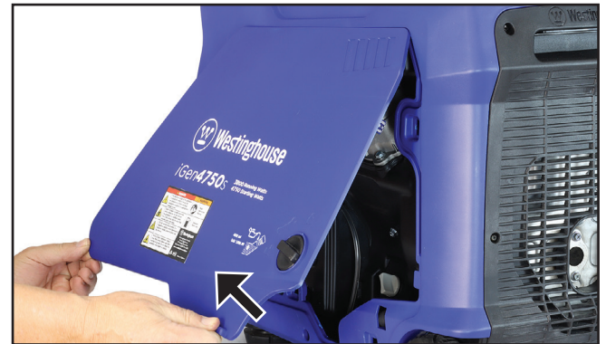
Figure 43 – Removing the RHS Maintenance Access Cover
