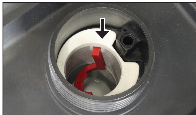
Figure 31 – Reinstalling the Fuel Strainer
