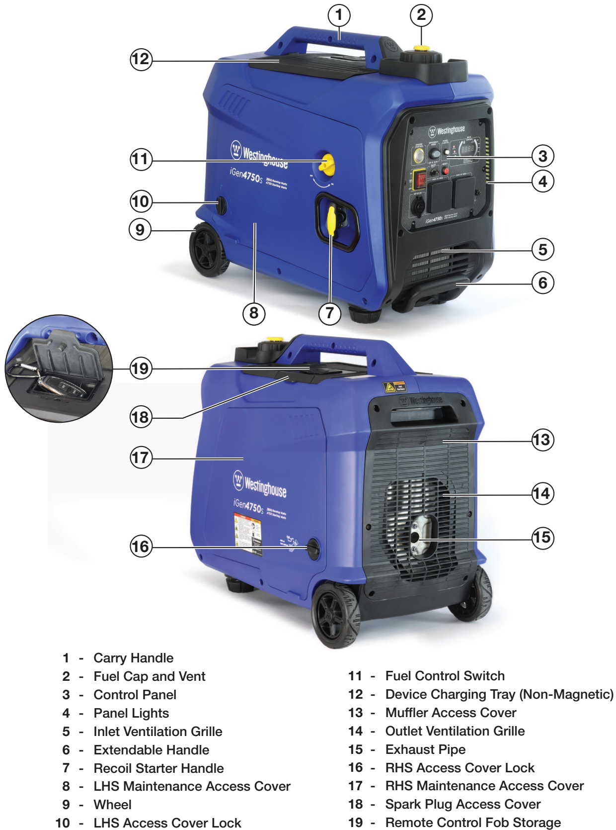
Figure 3 - iGen4750s Main Generator Components
